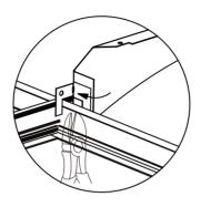
Use side cutters to adjust each tab to height of T-grid.
