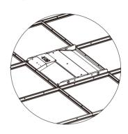
Lay fixture into T-grid.
