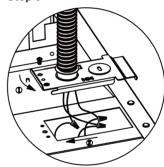
Ensure that the wiring of the last fixture in the row is properlyterminated. Then make all electrical connections to the fixture. Attach the wiring access cover plate.
