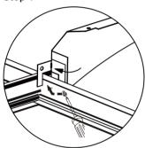
Bend tabs flush against T-grid in order to clear cornor for ceiling tile.
