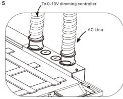
Plug in AC line(L and N,and GND) to the LED Driver using 18-14AWG Wire.When connecting 0-10Vdimming controller, wires must run through a separate knockout hole equipped with an appropriate electrical fitting.
