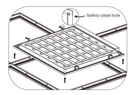
Insert luminaire into T-bar ceiling grid. Secure safety cable to connection hole as needed to meet local seismic requirements. Safety cable and method of attachment to the building provided by contractor according to local building codes.
