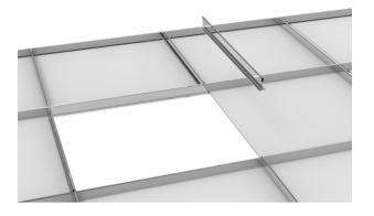
**STEP 5: SECURE THE T BAR LIGHT**Use a Phillips screwdriver to tight the clips on each end.
