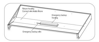
Mounting method 3: Emergency backup outside lighting without flexible conduit.
