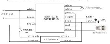
Note: Make sure the necessary branch circuit wiring is available. An unswitched source of power is required.
